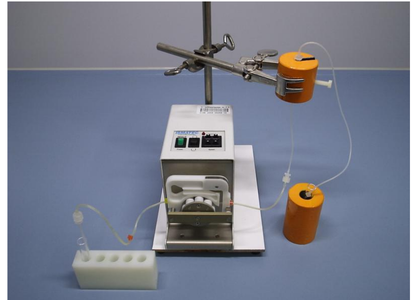
^{225}\text{Ac}/^{213}\text{Bi} generator in lead shielding with peristaltic pump for semiautomatic elution
